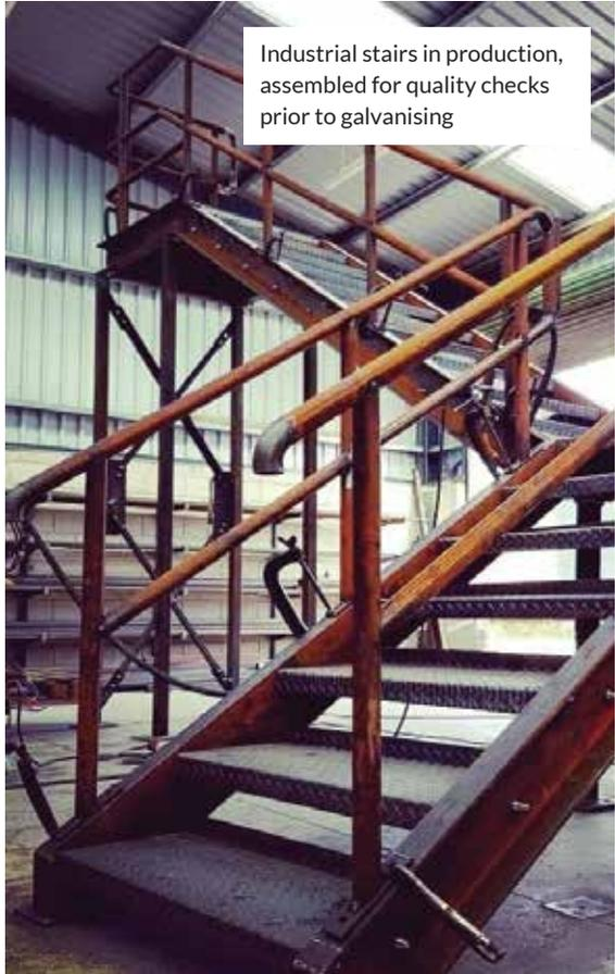
Industrial stairs in production, assembled for quality checks prior to galvanising
